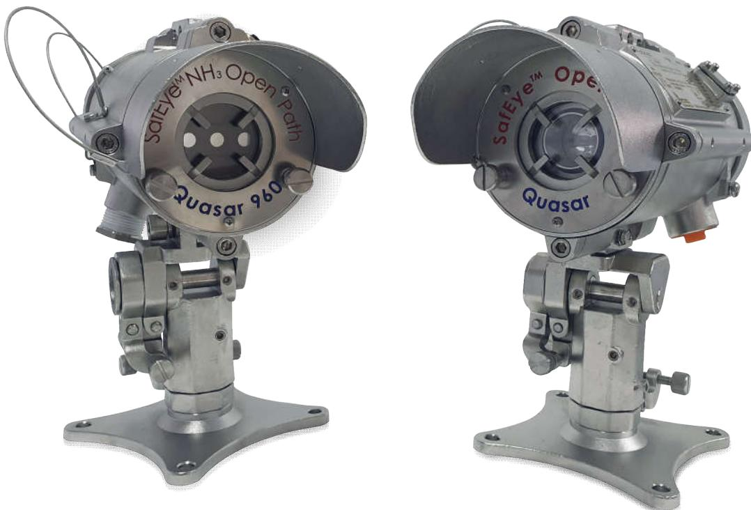
The SafEye Quasar 960 is part of the innovative SafEye Quasar open path gas detector series. The detector provides ultraviolet technology continuous monitoring for toxic ammonia ( $\text{NH}_3$ ) gas at very low concentrations, up to 95 percent obscuration, featuring advanced wide area coverage with long range detection up to 200 ft. (60 m) and high speed response in under 10 seconds.
